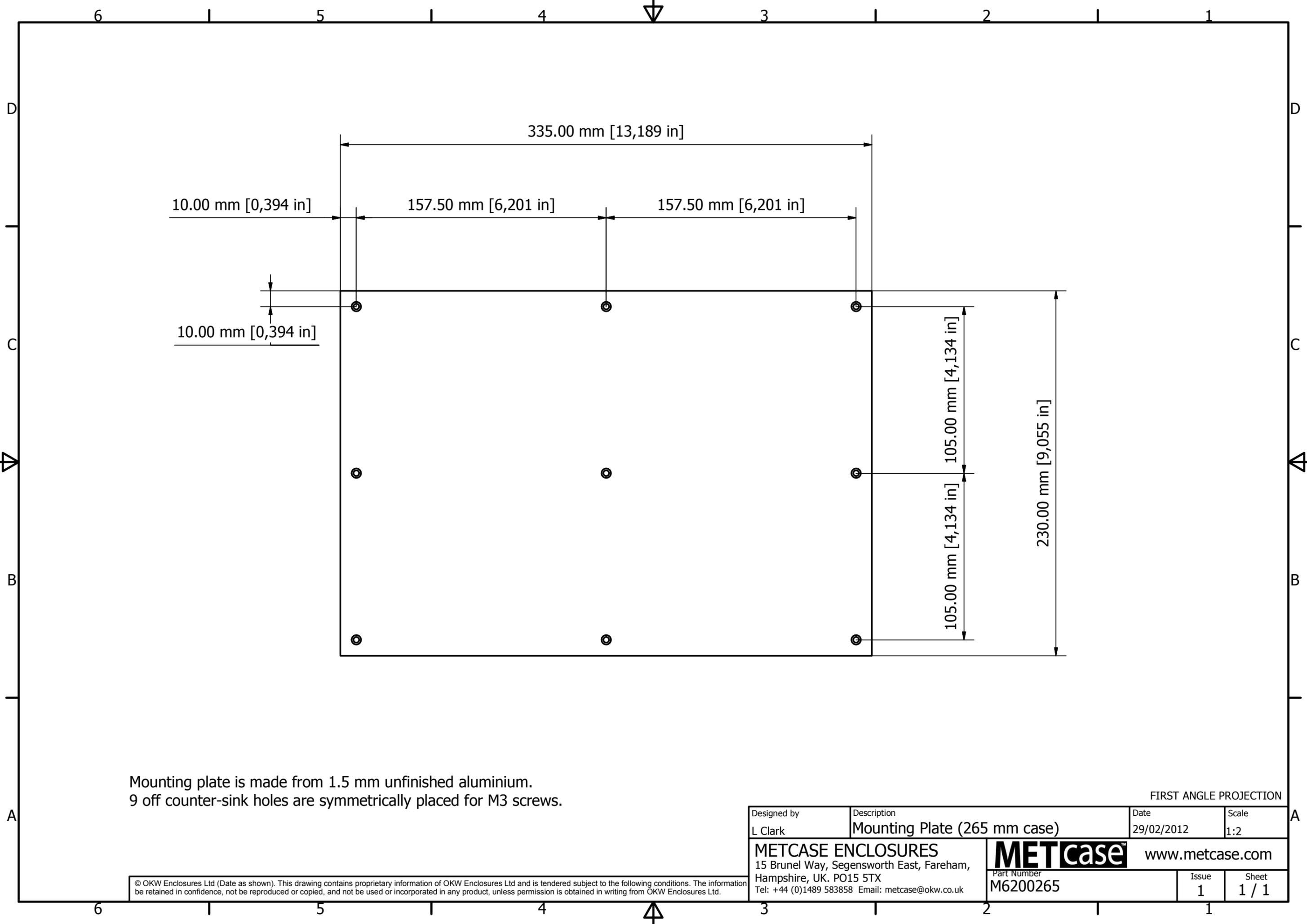
Mounting plate is made from 1.5 mm unfinished aluminium.
