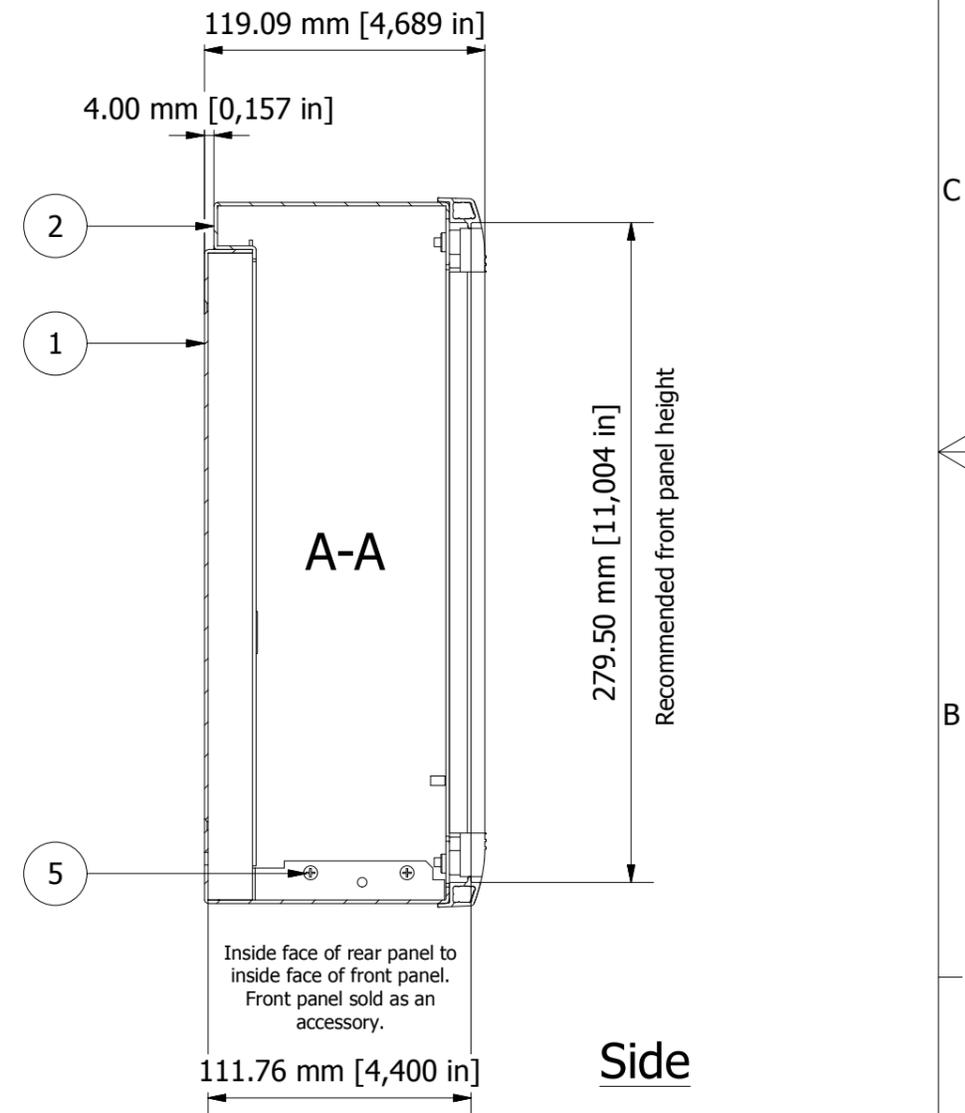
M3 countersink holes in rear panel for chassis plate / PCB mounting.
