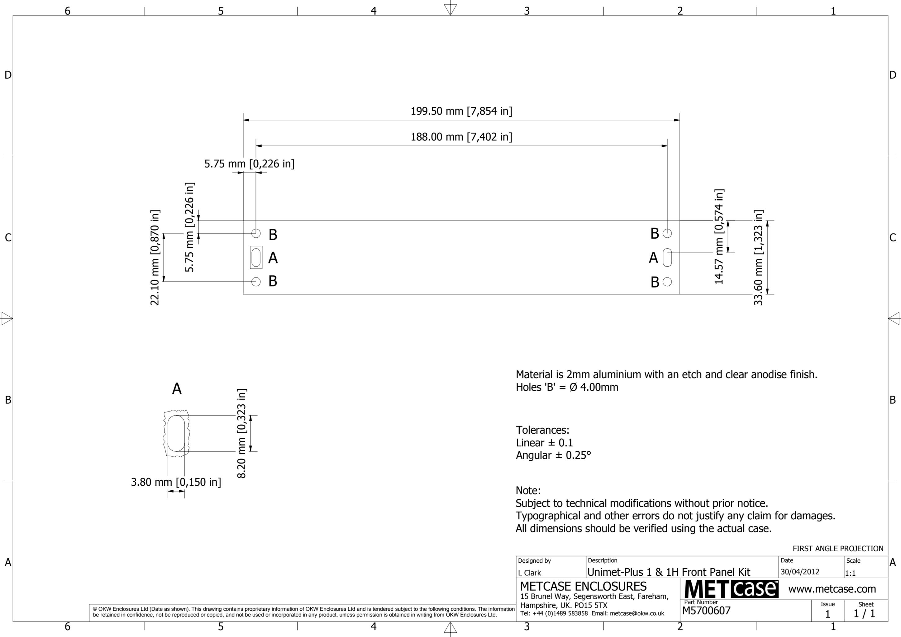
Material is 2mm aluminium with an etch and clear anodise finish.
